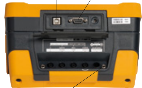
sockets to check 10 MOhm reference resistor
