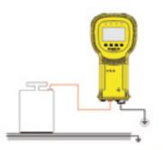
R<sub>g</sub>/R<sub>gp</sub> Resistance to ground or groundable point
